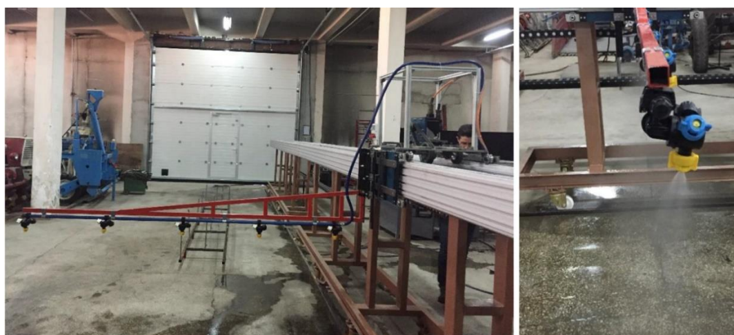
Figure 2. Spray boom and hydraulic nozzles
