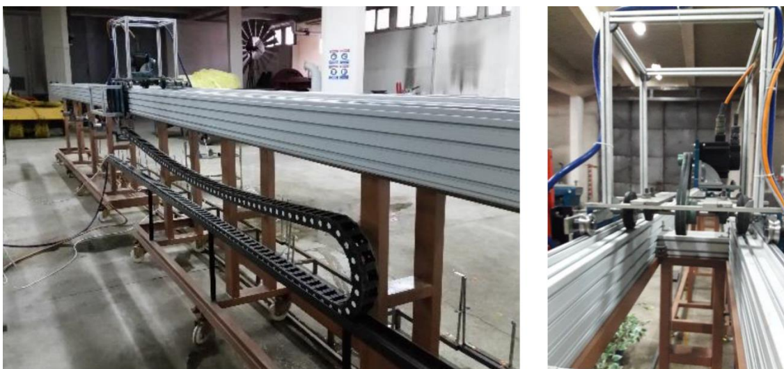
Figure 1. Spray simulator (a) rail of 12 meters (b) linear moving mechanism
