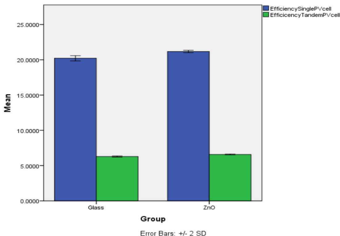
**Fig. 5.** The Bar chart compares mean (+/- 2 SD) efficiency of single junction PV cell and efficiency of tandem PV cell of Glass (protective layer) based solar cell and ZnO (protective layer) based solar cell by varying thickness. There is a significant difference between the two groups as  $p < 0.05$  (Independent Sample T Test). X Axis: Glass vs ZnO. Y Axis: Mean efficiency of Single PV cell and TandemPV cell.
