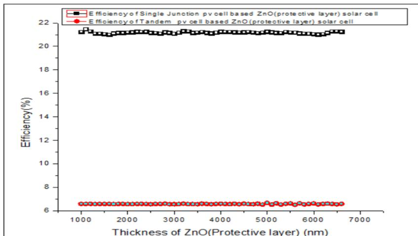
**Fig.2.** Comparison of efficiency for different PV cells in ZnO (protective layer) based solar cells. Efficiency is measured for varying protective layer thickness from 1000nm to 6600nm. Black line represents efficiency of single junction PV cell and red line represents efficiency of tandem PV cell. Single junction PV cell appears to have higher efficiency than tandem PV cell based ZnO (protective layer) based solar cell.
