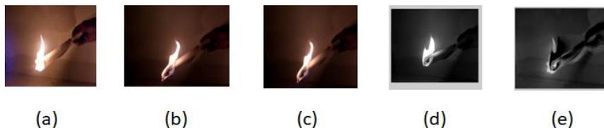
**Fig. 1.** Fire detection using frame difference method. (a) The input frame image. (b) The current frame image. (c) Image after thresholding. (d) Region of moving pixel. (e) The binary image after expansion
