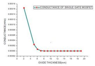
**Fig. 4.** Graphical representation of the conductivity of single gate MOSFET. Conductance and oxide thickness are found to be inversely proportional to each other.
