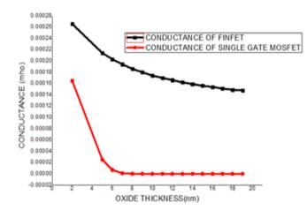
**Fig. 5.** Comparison of conductance of FinFET and MOSFET. Conductance of FinFET is found to be significantly better than single gate MOSFET.
