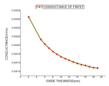
Fig. 2. Graphical representation of the conductivity of FinFET. Conductance of FINFIT appears to be inversely proportional to the thickness of the oxide layer.
