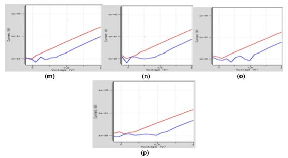
**Fig. 3.** Simulated IV characteristics of Single gate MOSFET for oxide thickness of (a) 2 nm (b) 5 nm (c) 6 nm (d) 7 nm (e) 8 nm (f) 9 nm (g) 10 nm (h) 11 nm (i) 12 nm (j) 13 nm (k) 14 nm (l) 15 nm (m) 16 nm (n) 17 nm (o) 18 nm (p) 19 nm. The red line represents the IV curve with a drain voltage of 1V and the blue line represents IV curve with a drain voltage of 0.05 V.
