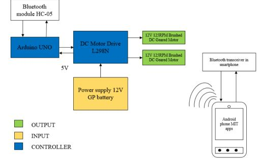
Figure 2. Showing the block diagram of the system
