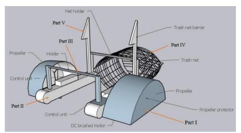
**Figure 9.** Showing the proposed design of garbage collector; propeller protector (Part I); control unit (Part II); robot rear parts connector (Part III); trash net (Part IV); trash barrier for preventing trash to come out (Part IV).
