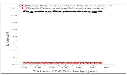
**Fig. 2.** Comparison of efficiency for different PV cells in ZnO (protective layer) based solar cells. Efficiency is measured for varying protective layer thickness from 1000nm to 6600nm. **Black** line represents efficiency of single junction PV cell and **red** line represents efficiency of tandem PV cell. Single junction PV cell appears to have higher efficiency than tandem PV cell based ZnO (protective layer) based solar cell.
