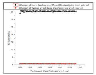
**Fig.1.** Comparison of efficiency for different PV cells in glass(Protective layer) based solar cell. Efficiency is measured for varying protective layer thickness from 1000nm to 6600nm. **Black** line represents efficiency of single junction PV cell and **red** line represents efficiency of tandem PV cell. Single junction PV cells appear to have higher efficiency than tandem PV cell glass(protective layer) based solar cells.
