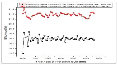
Fig.3. Comparison of efficiency of single junction PV cell based glass (protective layer) solar cell that is represented by black line and single junction PV cell based ZnO (protective layer) solar cell that is represented by red line.
