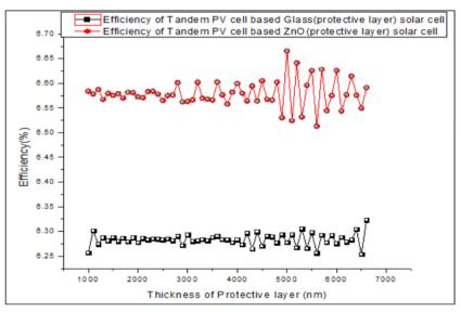
**Fig.4.** Comparison of efficiency of tandem PV cell based glass(protective layer) solar cell that is represented by **black** line and tandem PV cell based ZnO(protective layer) solar cell that is represented by **red** line. Efficiency of tandem PV cell based ZnO solar cells is higher compared to PV cell based glass solar cells.
