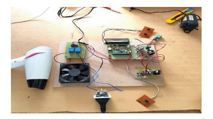
Here the circuit is turned ON by giving the regulated power supply of 12v which is converted to 5v dc current. The LED is the indication for 5v current so, if there is 5v current then automatically the LED glows. The generated 5v dc current passes to every hardware component in the circuit.
